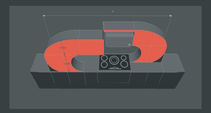
The minimum length (L) of the two curved modules is 2,50m. There is no maximum limit.
